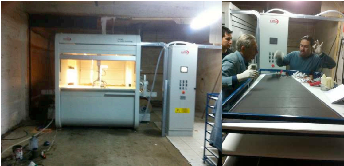
Figure 4. The left picture shows PRIMA/CELFA spraying/finishing machine ( https://www.ceflafinishing.com/en/products/product-search/prima-spraying-machine ) in the UTFSM Detector Laboratory, the machine was bought with FONDEQIP EQM 130244 (I was a director of this grant in 2014-2015). The right photo shows work on painted sTGC cathode.
