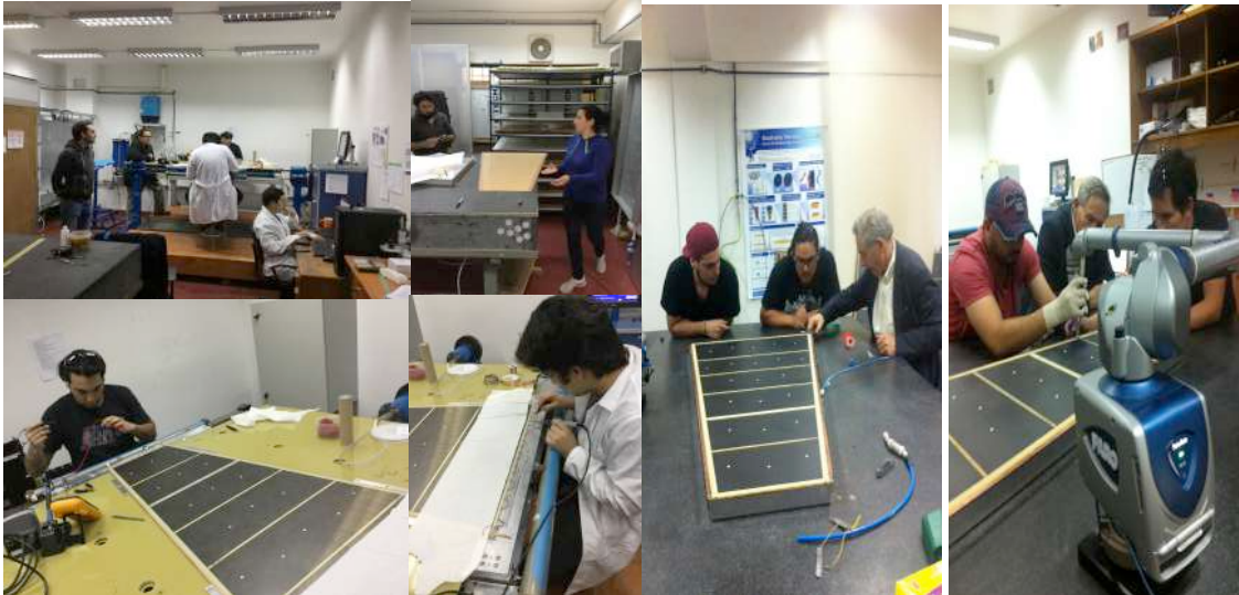
Figure 2. There are photos of my team technicians' working with my engineer, Rimsky Rojas, and my visitor, George Mikenberg in the sTGC production facility. Left photos show a work with the winding machine, the right photo shows a work with FARO ARM 3D position measurement system. It is possible to measure any 3D object with size 1.5x1.5x2. m 3 with 50 microns accuracy.
