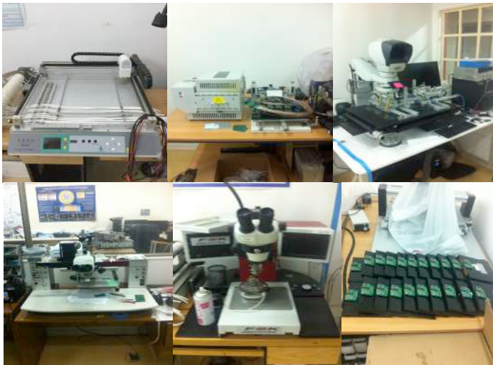
Figure 5. The electronic equipment of the microelectronic laboratory of the Detector Laboratory. A product of the laboratory, cosmic ray detectors (for schools and universities) are shown on left bottom picture. 400 such detectors were produced. 60 detectors were installed in the high energy physics laboratory in PUC (Santiago) for test of sTGC with cosmic ray.
